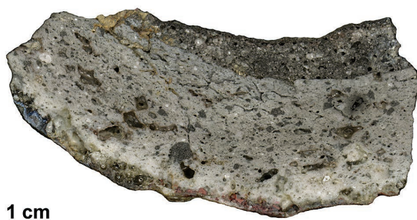
Figure 3: Section of crucible Fd. Nr. 3342 showing the two layered structure of the crucible and repair layer on the interior.
