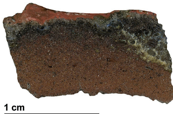
Figure 1: Section of open-faced crucible Fd. Nr. 410 with red glassy slag on the interior associated with dark vitrification of the ceramic. The ceramic is thoroughly burned and has a homogeneous texture (Keyence digital microscope image).
